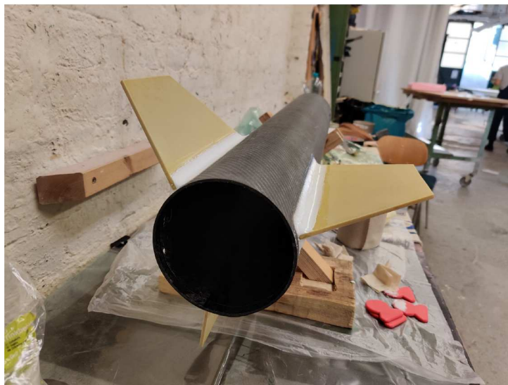
Figure 2.10: Applying the epoxy fillets
